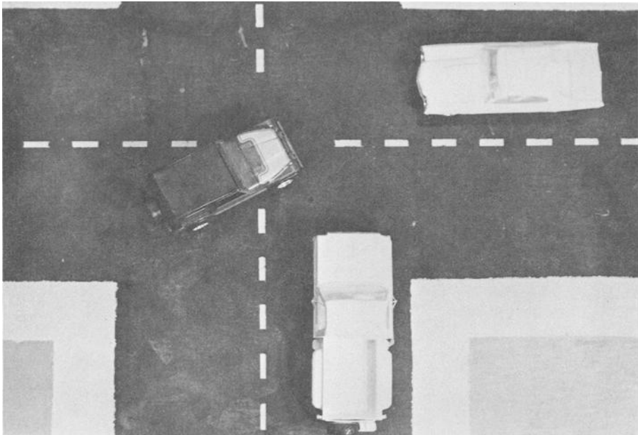
FIG. 3—A pickup truck, a full-sized car, and a four-wheel-drive vehicle are shown at a 1/25 th scale two-dimensional intersection. For reference, the spacing of the centerline markings is 25 mm (1 in.).
